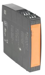
Dold safety relay extension module, 2-channel, 24 VAC/VDC, (7) N.O. safety output(s), (1) N.C. monitoring output(s), pluggable screw terminals.
