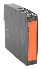
Dold safety relay extension module, 24 VAC/VDC, (5) N.O. safety output(s), (1) N.C. monitoring output(s), pluggable screw terminals.
