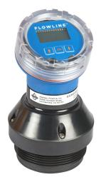
Flowline EchoPod reflective ultrasonic liquid level sensor, 39.3ft/12m sensing range, 4-20 mA, 14-28 VDC operating voltage, LCD digital display with pushbuttons, 3in male NPT process connection.
