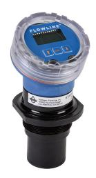
Flowline EchoPod reflective ultrasonic liquid level sensor, 19.6ft/6m sensing range, 4-20 mA, 14-28 VDC operating voltage, LCD digital display with pushbuttons, 2in male NPT process connection.
