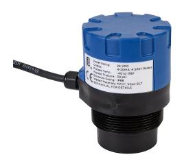
Flowline EchoPod reflective ultrasonic liquid level sensor, 9.8ft (3m) sensing range, 4-20 mA or (4) SPST relays, N.O./N.C. selectable, 14-28 VDC operating voltage, 2in male NPT process connection.
