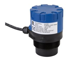
Flowline EchoPod reflective ultrasonic liquid level sensor, 4.9ft/1.5m sensing range, 4-20 mA and (4) SPST relays, N.O./N.C. selectable, 14-28 VDC operating voltage, 2in male NPT process connection.
