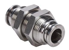
NITRA pneumatic push-to-connect fitting, bulkhead union, 316 stainless steel body, (1) 5/16in (8mm) push-to-connect to (1) 5/16in (8mm) push-to-connect.
