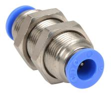
NITRA pneumatic push-to-connect fitting, bulkhead union, nickelplated brass body, (1) 6mm push-to-connect to (1) 6mm push-toconnect. Package of 5.
