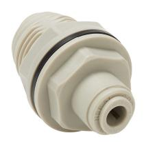
HydroMode potable water push-to-connect fitting, bulkhead union, acetal body, acetal threads, (1) 3/8in tube to (1) 1/4in tube connection(s), NSF/ANSI 61. Package of 5.
