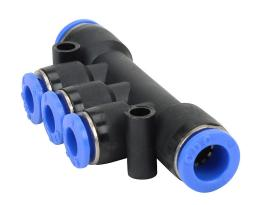
NITRA pneumatic push-to-connect fitting, union triple branch, thermoplastic (PBT) body, (2) 5/16in (8mm) push-to-connect to (3) 6mm push-to-connect. Package of 5.
