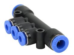
NITRA pneumatic push-to-connect fitting, union triple branch, thermoplastic (PBT) body, (2) 6mm push-to-connect to (3) 5/32in (4mm) push-to-connect. Package of 5.
