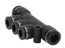
NITRA pneumatic push-to-connect fitting, union triple branch, thermoplastic (PBT) body, (2) 5/16in (8mm) push-to-connect to (3) 1/4in push-to-connect. Package of 5.
