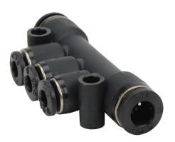
NITRA pneumatic push-to-connect fitting, union triple branch, thermoplastic (PBT) body, (2) 1/4in push-to-connect to (3) 5/32in (4mm) push-to-connect. Package of 5.
