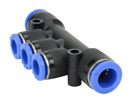
NITRA pneumatic push-to-connect fitting, union triple branch, thermoplastic (PBT) body, (2) 10mm push-to-connect to (3) 5/16in (8mm) push-to-connect. Package of 5.
