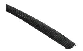
Iboco braided expandable sleeving, 0.75in nominal inside diameter, 0.63-1.37in stretching range, black, 164ft coil.
