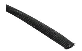
lboco braided expandable sleeving, 0.75in nominal inside diameter, 0.63-1.37in stretching range, black, 164ft coil.
