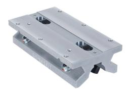
PBC TWN series twin roller pillow block, cam follower bearing, 6in overall length, steel, 1in inside diameter, aluminum housing, adjustable running clearance. For use with 1in diameter PBC shafts.
