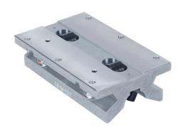
PBC TWN series twin roller pillow block, cam follower bearing, 4.5in overall length, steel, 3/4in inside diameter, aluminum housing, adjustable running clearance. For use with 3/4in diameter PBC shafts.
