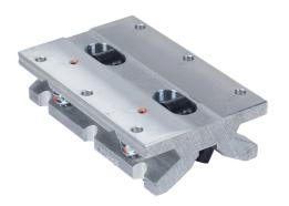
PBC TWN series twin roller pillow block, cam follower bearing, 4in overall length, steel, 5/8in inside diameter, aluminum housing, adjustable running clearance. For use with 5/8in diameter PBC shafts.
