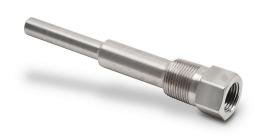
ProSense thermowell, 1/2in female NPT probe connection, 3/4in male NPT process connection, 316 stainless steel body, 12-1/4in overall length, 0.260in bore.
