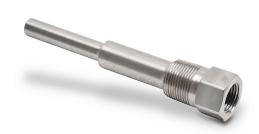
ProSense thermowell, 1/2in female NPT probe connection, 3/4in male NPT process connection, 304 stainless steel body, 12-1/4in overall length, 0.260in bore.
