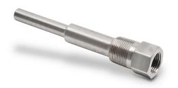
ProSense thermowell, 1/2in female NPT probe connection, 3/4in male NPT process connection, 304 stainless steel body, 12-1/4in overall length, 0.260in bore.
