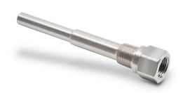
ProSense thermowell, 1/2in female NPT probe connection, 1/2in male NPT process connection, 304 stainless steel body, 12-1/4in overall length, 0.260in bore.
