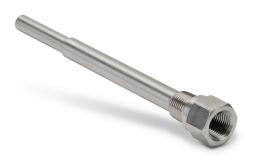
ProSense thermowell, 1/2in female NPT probe connection, 1/2in male NPT process connection, 316 stainless steel body, 9-1/4in overall length, 0.260in bore.
