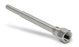
ProSense thermowell, 1/2in female NPT probe connection, 1/2in male NPT process connection, 304 stainless steel body, 9-1/4in overall length, 0.260in bore.
