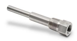
ProSense thermowell, 1/2in female NPT probe connection, 3/4in male NPT process connection, 316 stainless steel body, 6-1/4in overall length, 0.260in bore.
