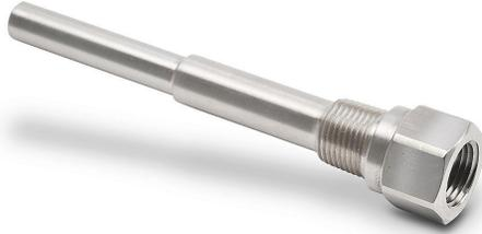
ProSense thermowell, 1/2in female NPT probe connection, 1/2in male NPT process connection, 316 stainless steel body, 6-1/4in overall length, 0.260in bore.
