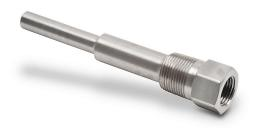
ProSense thermowell, 1/2in female NPT probe connection, 3/4in male NPT process connection, 304 stainless steel body, 6-1/4in overall length, 0.260in bore.
