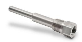
ProSense thermowell, 1/2in female NPT probe connection, 3/4in male NPT process connection, 304 stainless steel body, 6-1/4in overall length, 0.260in bore.
