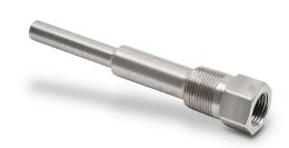
ProSense thermowell, 1/2in female NPT probe connection, 3/4in male NPT process connection, 316 stainless steel body, 4-1/4in overall length, 0.260in bore.
