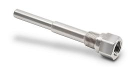
ProSense thermowell, 1/2in female NPT probe connection, 1/2in male NPT process connection, 316 stainless steel body, 4-1/4in overall length, 0.260in bore.
