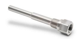
ProSense thermowell, 1/2in female NPT probe connection, 1/2in male NPT process connection, 316 stainless steel body, 4-1/4in overall length, 0.260in bore.
