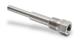
ProSense thermowell, 1/2in female NPT probe connection, 3/4in male NPT process connection, 304 stainless steel body, 4-1/4in overall length, 0.260in bore.
