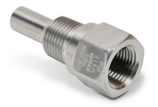
ProSense thermowell, 1/2in female NPT probe connection, 1/2in male NPT process connection, 316 stainless steel body, 2-3/4in overall length, 0.260in bore.
