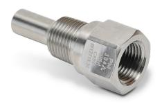
ProSense thermowell, 1/2in female NPT probe connection, 1/2in male NPT process connection, 304 stainless steel body, 2-3/4in overall length, 0.260in bore.
