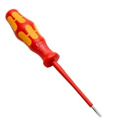
Wera Kraftform Plus 2.5mm slotted insulated screwdriver, 1000V insulation rating, 3.1in (80mm) shaft length, Kraftform ergonomic handle.
