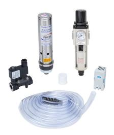
Stratus vortex cooler kit, 1800 BTUH (528W), 25 SCFM (708 SLPM), 120 VAC operating voltage, stainless steel body. For use with NEMA 4, NEMA 4X and NEMA 12 enclosures.
