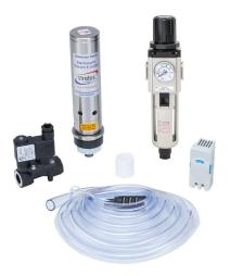
Stratus vortex cooler kit, 1000 BTUH (293W), 15 SCFM (425 SLPM), 24 VDC operating voltage, stainless steel body. For use with NEMA 4, NEMA 4X and NEMA 12 enclosures.
