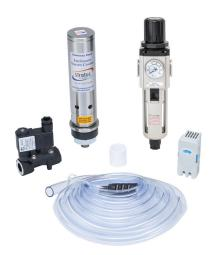
Stratus vortex cooler kit, 1000 BTUH (293W), 15 SCFM (425 SLPM), 24 VDC operating voltage, stainless steel body. For use with NEMA 4, NEMA 4X and NEMA 12 enclosures.
