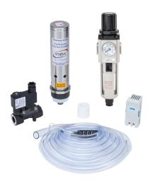
Stratus vortex cooler kit, 1000 BTUH (293W), 15 SCFM (425 SLPM), 120 VAC operating voltage, stainless steel body. For use with NEMA 4, NEMA 4X and NEMA 12 enclosures.
