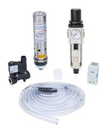
Stratus vortex cooler kit, 600 BTUH (176W), 10 SCFM (283 SLPM), 24 VDC operating voltage, stainless steel body. For use with NEMA 4, NEMA 4X and NEMA 12 enclosures.
