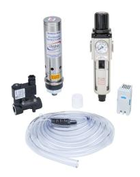
Stratus vortex cooler kit, 600 BTUH (176W), 10 SCFM (283 SLPM), 120 VAC operating voltage, stainless steel body. For use with NEMA 4, NEMA 4X and NEMA 12 enclosures.
