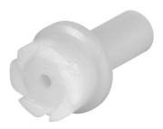
Stratus vortex generator, replacement, 500 BTUH (147W), 8 SCFM (227 SLPM), polypropylene, white. For use with all Stratus vortex coolers.
