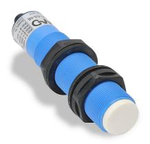
Micro Detectors ultrasonic proximity sensor, tubular, 30mm diameter x 124mm body, polybutylene terephthalate housing, PNP, N.O. output, 300-2500mm sensing distance, 1 Hz switching frequency, IP67, 4-pin M12 quick-disconnect.
