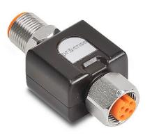
ProSense temperature transmitter, isolated, Pt100 RTD input, -40 to 300 deg F fixed, 4-20 mA output, 20-32 VDC operating voltage, M12 in-line mount, 4-pin M12 quick-disconnect.
