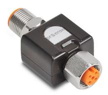
ProSense temperature transmitter, isolated, Pt100 RTD input, -40 to 300 deg F fixed, 4-20 mA output, 20 to 32 VDC operating voltage, M12 in-line mount, 4-pin M12 quick-disconnect.
