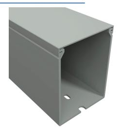
Iboco TSH series solid wire duct, 2.25in width, 3in height, 6.5ft/2m length, gray. Cover included.
