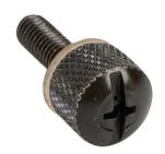
Hammond thumb screw, #10-32 UNF x 0.625in, Phillips/slotted combo knurled head, carbon steel, black oxide finish. Package of 25. Nylon washer included.
