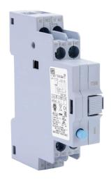
WEG Electric field installable short circuit alarm contact, left side mount, (2) N.O./(2) N.C. contact(s), 6A @ 120 VAC/0.55A @ 120 VDC, screw terminal. For use with MPW40 and MPW80 series manual motor protectors.
