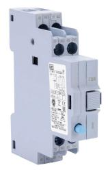
WEG Electric field installable short circuit alarm contact, left side mount, (2) N.O./(2) N.C. contact(s), 6A @ 120 VAC/0.55A @ 120 VDC, screw terminal. For use with MPW40 and MPW80 series manual motor protectors.
