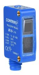
Contrinex photoelectric sensor, rectangular, polarized retroreflective, ultra violet light emission, 1m sensing distance, complementary light-on/dark-on, PNP, teach-in button, 4-wire, 4-pin M8 quick-disconnect.
