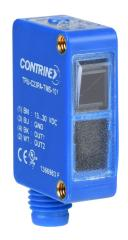
Contrinex photoelectric sensor, rectangular, polarized retroreflective, ultra violet, 1m sensing distance, complementary light-on/dark-on, NPN, teach-in button, 4-wire, 4-pin M8 quick-disconnect.
