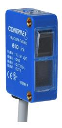
Contrinex photoelectric sensor, rectangular, polarized retroreflective, ultra violet light emission, 1m sensing distance, complementary light-on/dark-on, PNP, teach-in button, 4-wire, pigtail.
