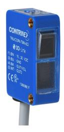
Contrinex photoelectric sensor, rectangular, polarized retroreflective, ultra violet, 1m sensing distance, complementary light-on/dark-on, PNP, teach-in button, 4-wire, pigtail.
