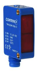
Contrinex photoelectric sensor, rectangular, polarized retroreflective, visible red light emission, 20-4200mm sensing distance, complementary light-on/dark-on, NPN, teach-in button, 4-wire, 4-pin M8 quick-disconnect.
