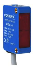
Contrinex photoelectric sensor, rectangular, polarized retroreflective, visible red, 20-4200mm sensing distance, complementary light-on/dark-on, PNP, teach-in button, 4-wire, pigtail.
