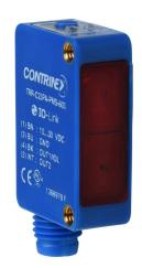
Contrinex photoelectric sensor, rectangular, polarized retroreflective, visible red light emission, 20-4200mm sensing distance, complementary light-on/dark-on, PNP, potentiometer, 4-wire, 4-pin M8 quick-disconnect.
