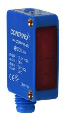
Contrinex photoelectric sensor, rectangular, polarized retroreflective, visible red, 20-4200mm sensing distance, complementary light-on/dark-on, PNP, potentiometer, 4-wire, 4-pin M8 quick-disconnect.
