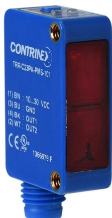
Contrinex photoelectric sensor, rectangular, polarized retroreflective, visible red, 20-4200mm sensing distance, complementary light-on/dark-on, NPN, potentiometer, 4-wire, 4-pin M8 quick-disconnect.
