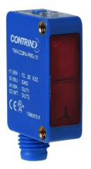
Contrinex photoelectric sensor, rectangular, polarized retroreflective, visible red, 20-4200mm sensing distance, complementary light-on/dark-on, NPN, potentiometer, 4-wire, 4-pin M8 quick-disconnect.
