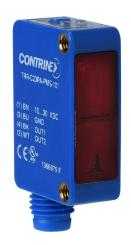
Contrinex photoelectric sensor, rectangular, polarized retroreflective, visible red light emission, 20-4200mm sensing distance, complementary light-on/dark-on, NPN, potentiometer, 4-wire, 4-pin M8 quick-disconnect.
